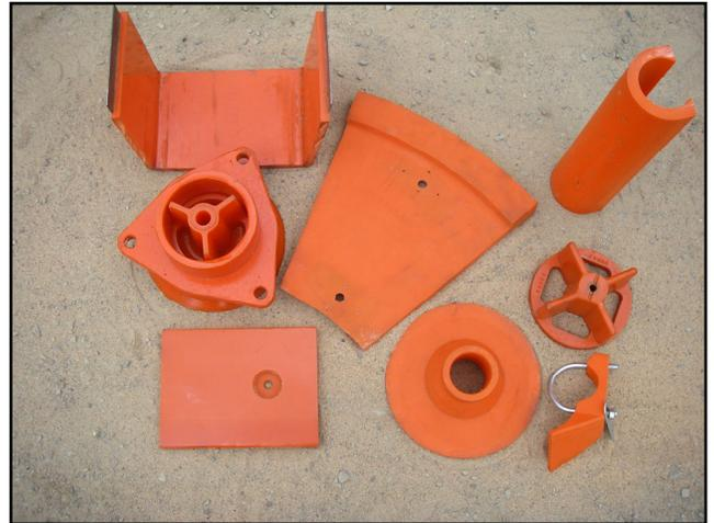
Durex® manufacturers made to order liners for feed boxes, discharge lips and chutes with several ways to install.
