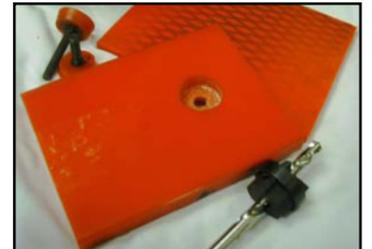
Liners can be supplied with urethane coated bolts for ½" and thicker sheets. These bolts are tapered for a tight fit into counter bored holes. The tight fit allows the bolts to be tightened from the back without turning.
