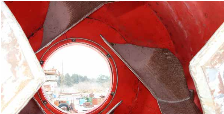
Magnetic and Weldable Mixer Liner Set: Reduces installation and eventual removal of the liners. Also, concrete flows smoothly over liners with fewer plug-weld indentations, causing less turbulence and, thus, less wear.
