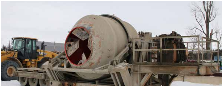
Magnetic and Weldable Mixer Liner Set: Reduces installation and eventual removal of the liners. Also, concrete flows smoothly over liners with fewer plug-weld indentations, causing less turbulence and, thus, less wear.
